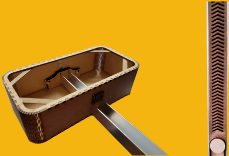
Figure 8. Construction of the camera and covering the ledstrip with lasercut wood
